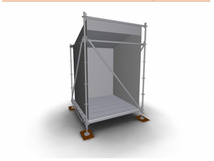
The Core-a-sol is a waterproof PVC cover to protect light and sound equipment at a festival from rain and beer showers. The cover is simply hung up in the scaffolding structure with four lashing straps and then forms a 'tent' with a floor space of  $1.90 \times 1.90$  metres. At the front the cover is 2.5 metres high and at the back 2 metres high. The front flap can be zipped open and rolled up.
