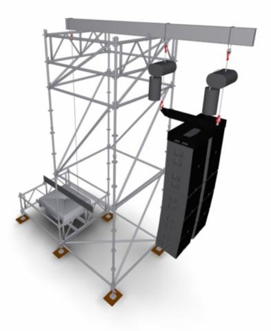
Fixed aluminum hoisting beam, 4,5 meters long. Intended for hanging light-weight PA systems on the outside of the <u>tower</u> <u>construction</u>. The alu beam is less heavy than the steel hoisting beam, and can be mounted on the tower manually. The <u>ballast</u> lies at the back of the construction.
